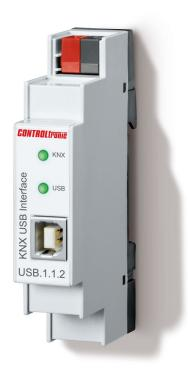
The KNX USB Interface is a data interface between a PC or notebook and the KNX bus. It can be used as a programming interface for ETS and supports KNX long frames. Long telegrams enable a faster download to devices supporting long frames.
